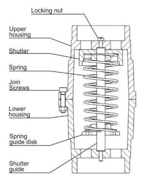
BLSV valves are used to limit pressure or vacuum on lateral channel blowers. When the pressure or vacuum is reached the valve opens and, connecting the internal part of blower to atmosphere, prevents to overcome the blower design limit. The discharge connection may be, according to the plant design, opened to atmosphere directly or channeled to a discharge pipe.
